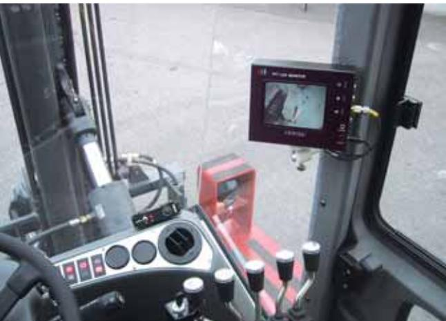
**A wireless camera system improves sawmill operation.**
